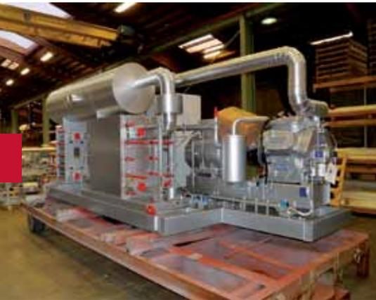
The compact NH3 heat pump after the test run at the factory
