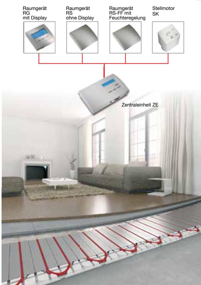
Underfloor heating systems in houses with a high level of thermal insulation often respond too late to interior and exterior heat gains. The autoadaptive individual room controller from Thermozyklus with its AA eu.bac product certification achieves a CA value of 0.5 K.
